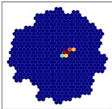
The data detected by the telescope's camera form "images" of the air shower
