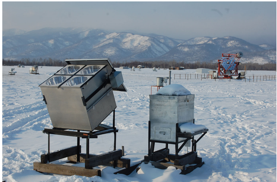
Fig. 24 One of the TAIGA-HiSCORE integrating Cherenkov detector stations with a wide Field of View is seen at the front in the above photograph. Each detector station consists of 4 large area PMTs. One installed TAIGA-IACT telescope seen at the back. Picture courtesy: TAIGA Collaboration
