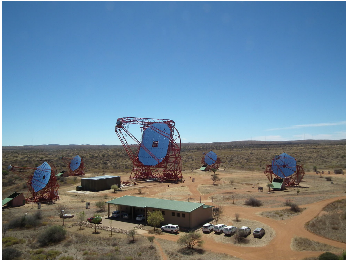
Fig. 9 H.E.S.S. IACT array at GAMESBERG in Namibia, consisting of four 12-m-diameter and one 28-m-diameter telescope. Picture courtesy: H.E.S.S. collaboration
